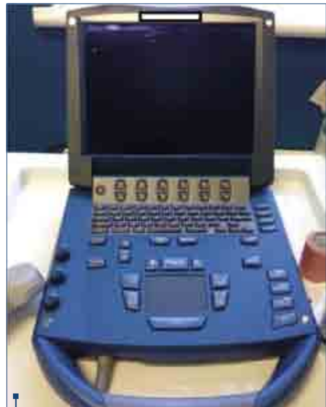
Figure 2. Portable ultrasound machine and abdominal probe, curvilinear transducer, 2-5 MHz, suitable for thoracic ultrasound
